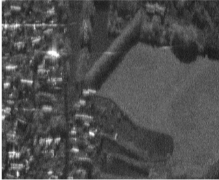
Figure 9: Resulting scene after processing with motion compensation (cut-out)
