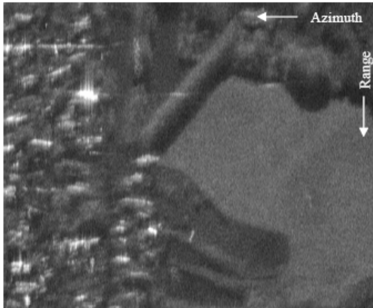
Figure 8: Resulting scene after processing without motion compensation (cut-out)
